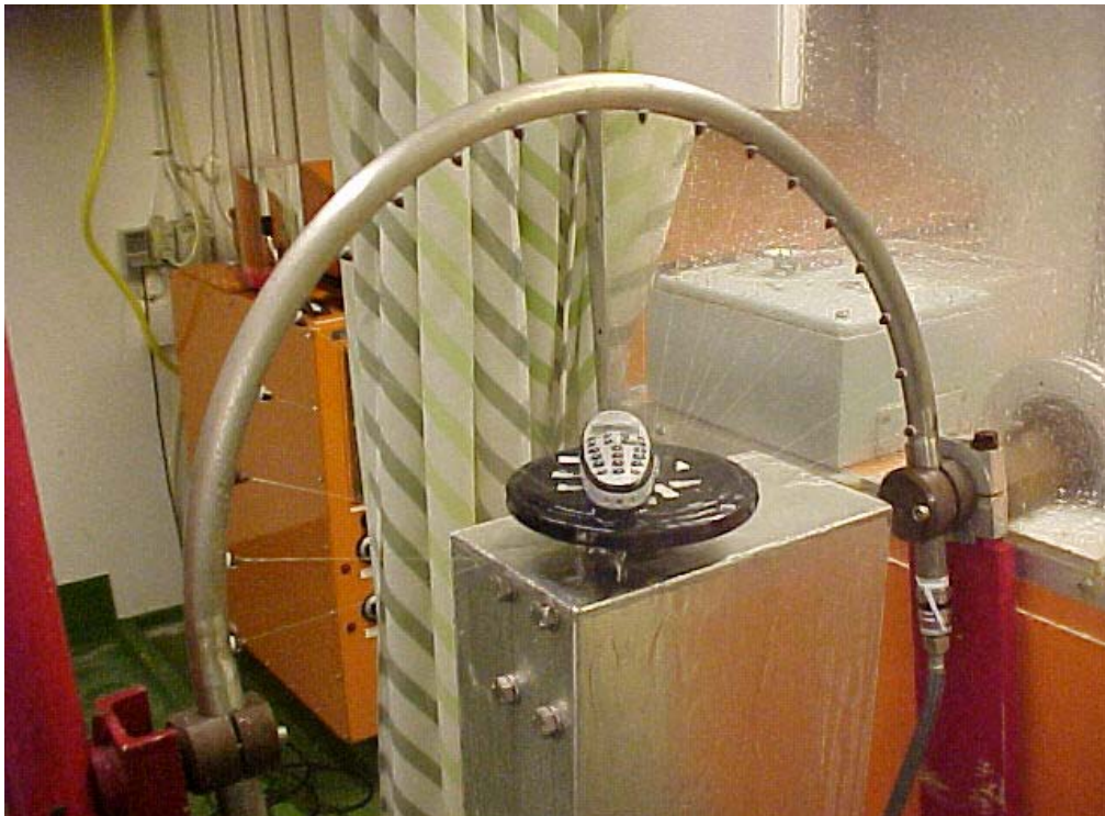
PHOTO 10. Test set-up enclosure protection testing (splashing).
