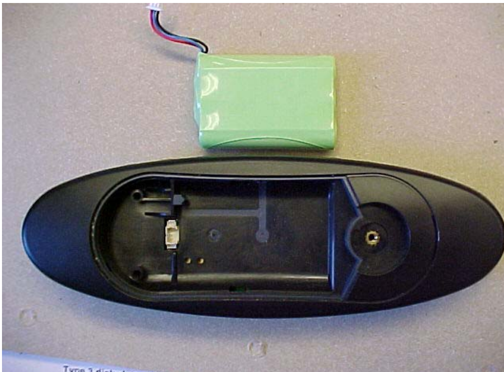
PHOTO 4. Visual inspection after salt mist testing (no salt deposits inside).
