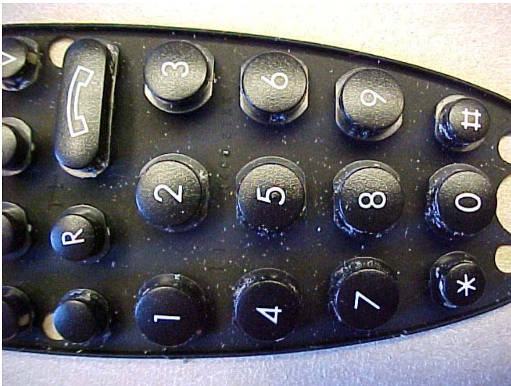
PHOTO 6. Small amount of salt deposits on keyboard membrane (external side).
