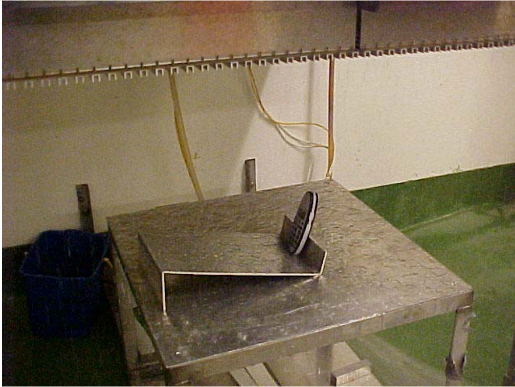
PHOTO 7. Test set-up enclosure protection testing (dripping).
