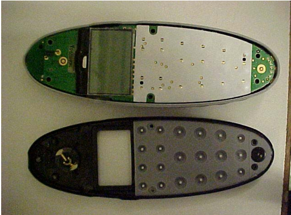
PHOTO 11. Visual inspection after splashing (one drop observed under keyboard membrane).
